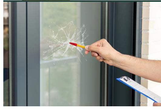
While this product cannot be sold as bulletproof, the glass all held in place, and we could not gain access. For this test, I also used a mirrored tinted security film; this prevents an intruder from seeing in from the outside, adding an additional level of security for your home or business.
